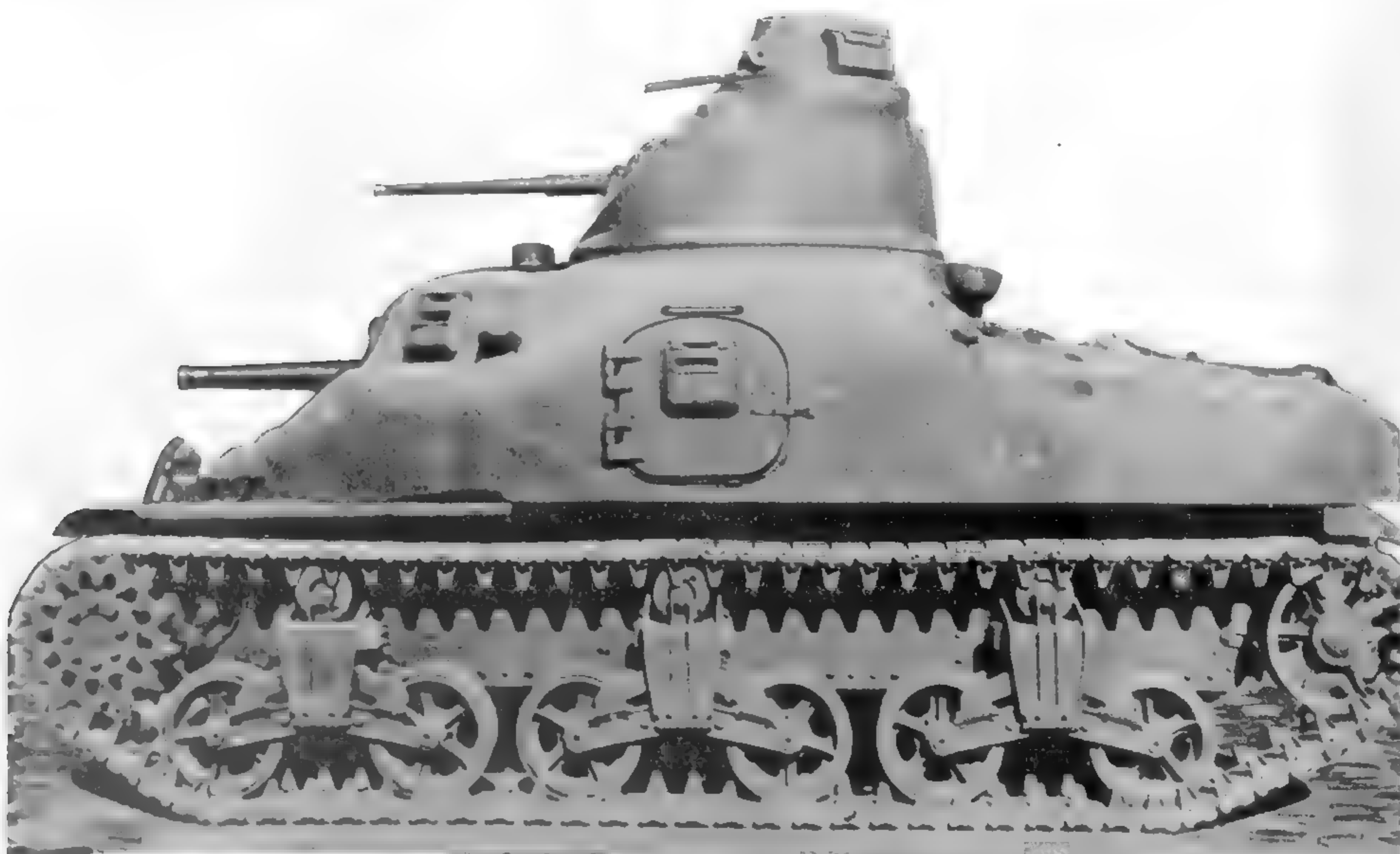
The M3A1 had a much smoother-cast hull than the M3. This was also much safer for the crews, who were sometimes injured when rivet heads were sheared off by enemy fire, allowing the rivets to fly about the interior of the tank. (Photo courtesy of the Patton Museum)
